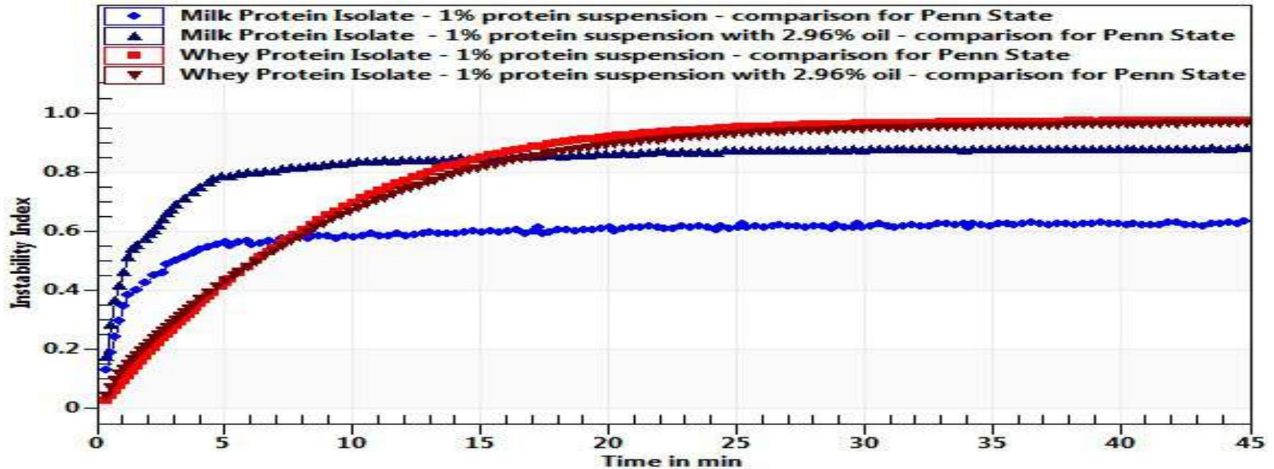
Note: - test solutions standardized to 1% protein with 2.96% corn oil - HTST processed, unhomogenized - 5° C overnight - 4000 RPM at 5°C - 45 minutes
