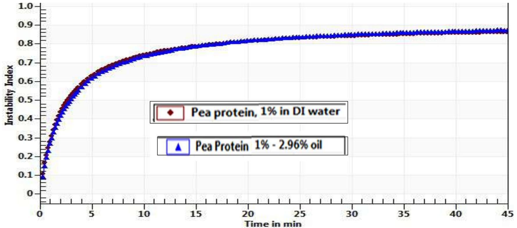
Note: - test solutions standardized to 1% protein with 2.96% corn oil - HTST processed, unhomogenized - 5° C overnite – 4000 RPM at 5°C – 45 minutes
