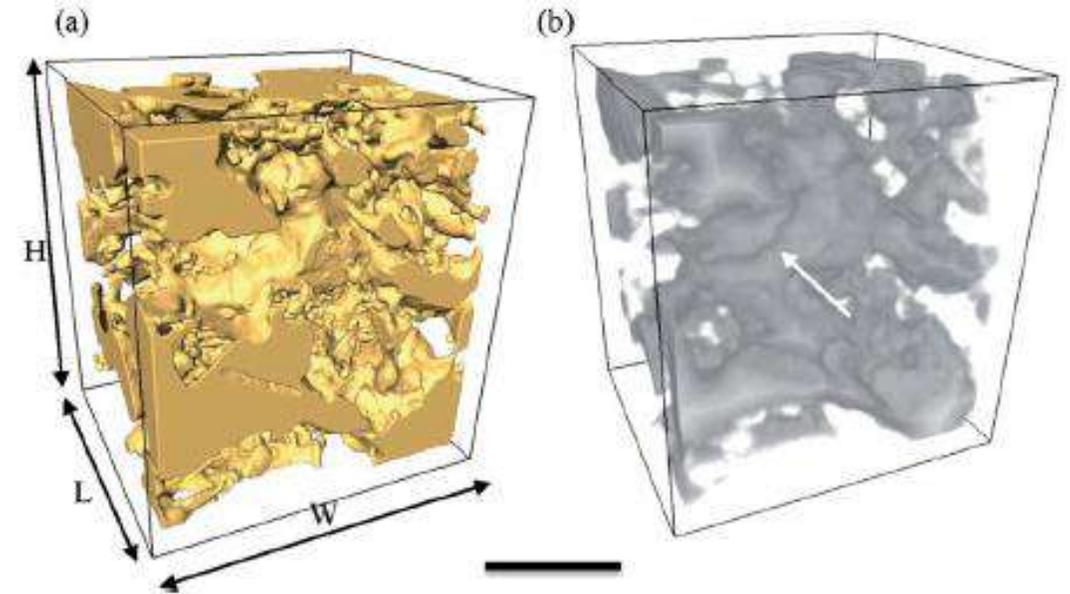
Fig. 8 3D image of an air cell channel in the C<sub>14</sub> ice cream sample: (a) isosurface 3D rendering, (b) skeleton of the air cells showing a channeling feature. Volume box size is  $545 \times 416 \times 499$  ( $H \times L \times W$ )  $\mu\text{m}^3$ . Scale bar is 200  $\mu\text{m}$  for both images.
