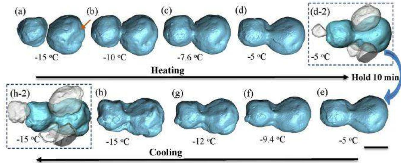
Fig. 9. Coalescence of two air cells during the heating stage (a–d) and cooling stage (e–h) of a thermal cycle. (d-2) and (h-2) show the morphological relationship between the surrounding ice crystals and the air cell at  $-5\text{ }^{\circ}\text{C}$  and  $-15\text{ }^{\circ}\text{C}$ , respectively. Scale bar  $100\text{ }\mu\text{m}$  for all images.
