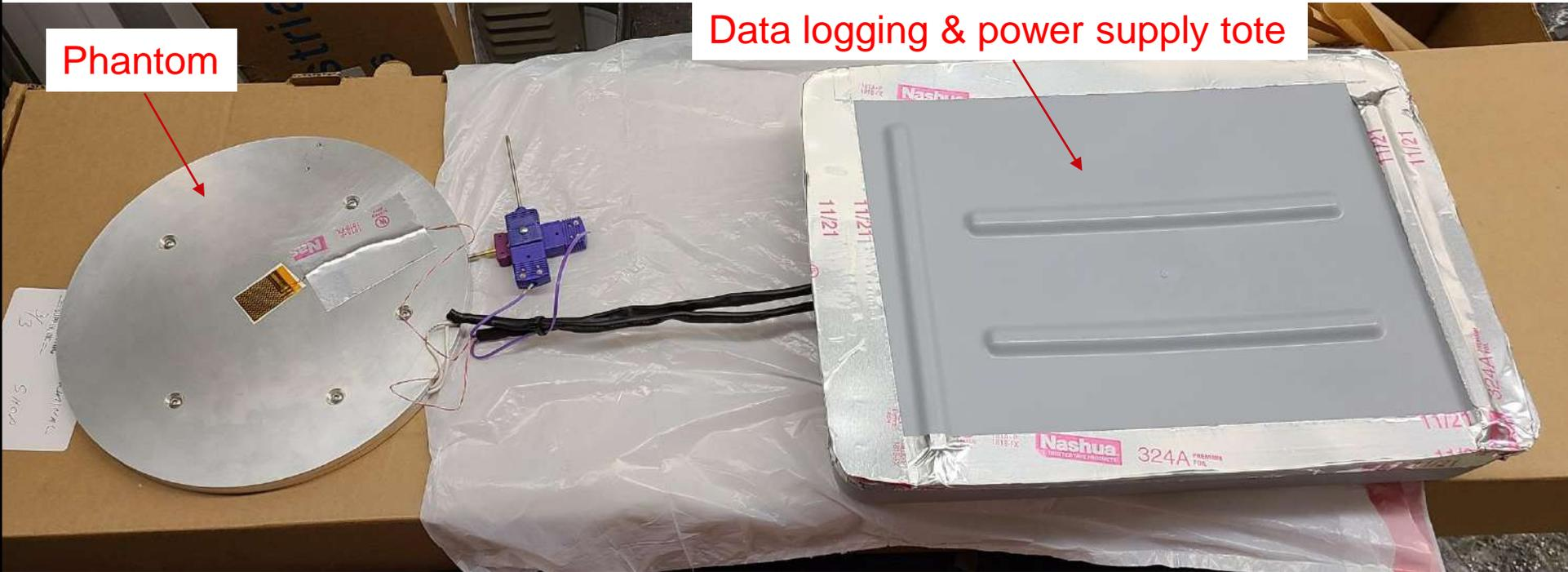
The Phantom is an instrument that simulates the product being frozen for the purpose of gathering heat transfer data within the operating blast freezing system
